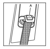
To move it down, press the release button (A) and move the height adjuster to the desired position. You can move the height adjuster up just by pushing up on the shoulder belt guide.
